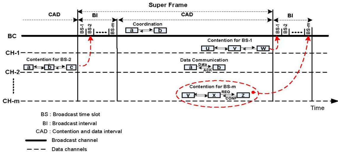
Fig 1. Super frame structure.
