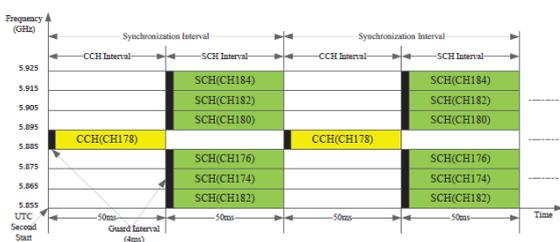
Fig. 1: Frequency channel layout of a 5.9GHz WAVE system.
