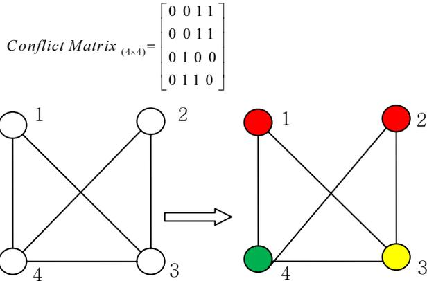
We can transmit link 1, 2 in the first timeslot, link 3 in the second timeslot and link 4 in the third timeslot.
