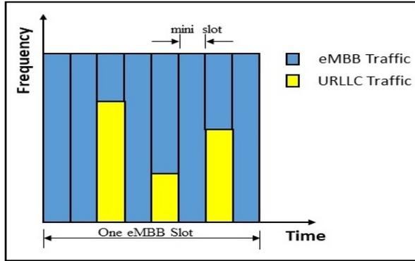
Figure 1: Puncturing approach for multiplexing of URLLC and eMBB
