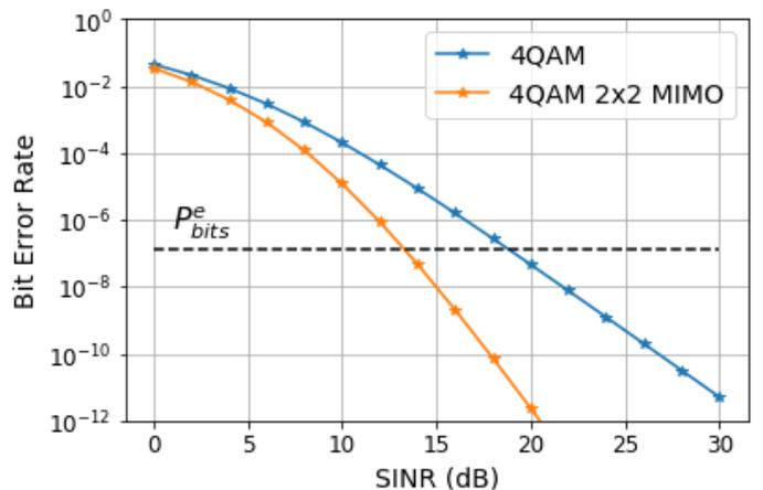
Fig. 3: BER of 4-QAM modulation with orthogonal STBC over exponentially correlated Rayleigh fading MIMO channels as a function of SINR
