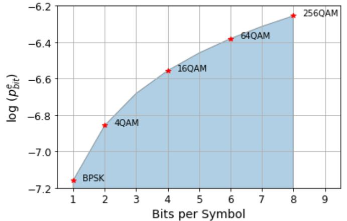
Fig. 2: Bit error rate versus bits per symbol
