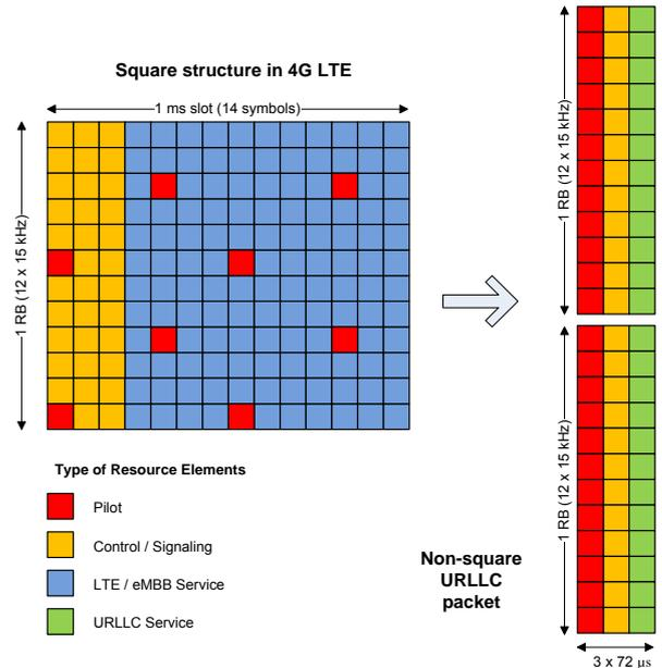
Fig. 1: LTE frame structure versus URLLC packet [1].
