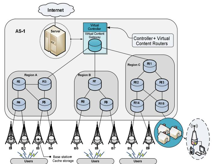
Figure 1 NFV deployment on CCN architecture
