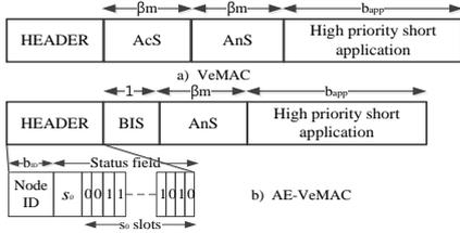
Fig. 3: Format of each packet transmitted on the CCH.
