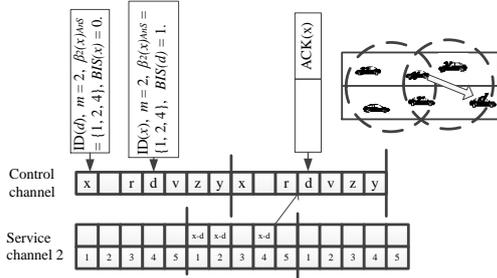
Fig. 4: Operation of AE-VeMAC protocol.
