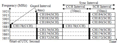
Fig. 1: Frequency channel layout of a 5.9GHz WAVE systems.
