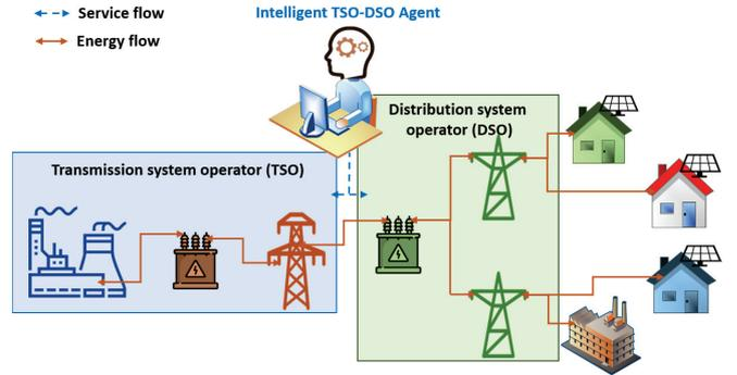
Figure 1: A system model for coordinating between TSO and DSO by an intelligent agent for a stable energy market.
