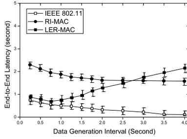
Fig. 8. Average End-to-End Latency varying Data Generation Interval
