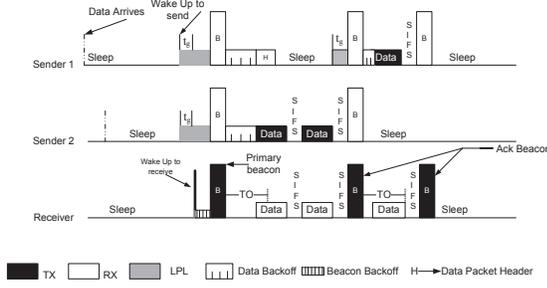
Fig. 2. The value of  $N_r$  is set as 3 as for example. Sender 2 wins the channel but have only 2 packets in the queue. It goes to sleep after transmitting all the packets in its queue. Sender 1 overhears the first packet header of sender 2 and then goes to sleep. It wakes up again with a guard time and sends the remaining number of packets in that reception round and goes to sleep again.
