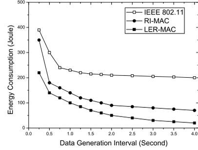
Fig. 7. Energy Consumption varying Data Generation Interval
