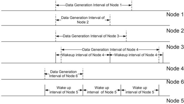
(b) Wake-up interval of node 4 and node 5. Node 4 updates its wake-up interval as equal as data generation interval of node 2 (the minimum interval among node 1, 2, 3 and 4). Similarly node 5 updates its wake-up interval as node 6's data generation interval.
