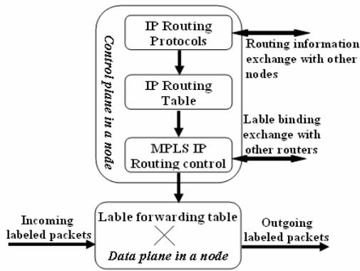
Figure 1. Basic Architecture of an MPLS Node Performing IP Routing.
