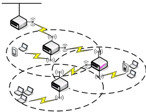
Figure 2. Three-radio MRs in Wireless Mesh Network.
