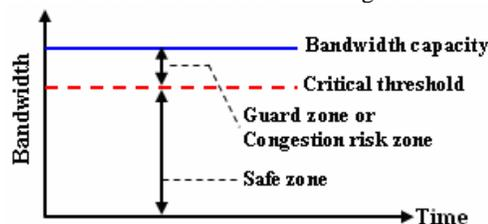
Figure 6. Proposal link selection mechanism based on critical threshold.
