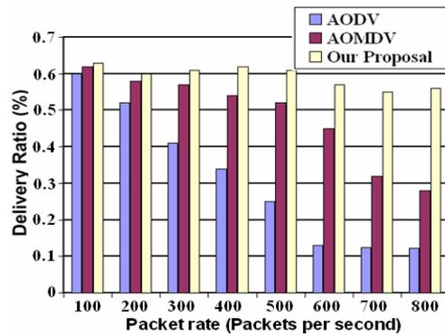
Figure 9. The delivery ratio analysis in comparison with AODV and AOMDV.
