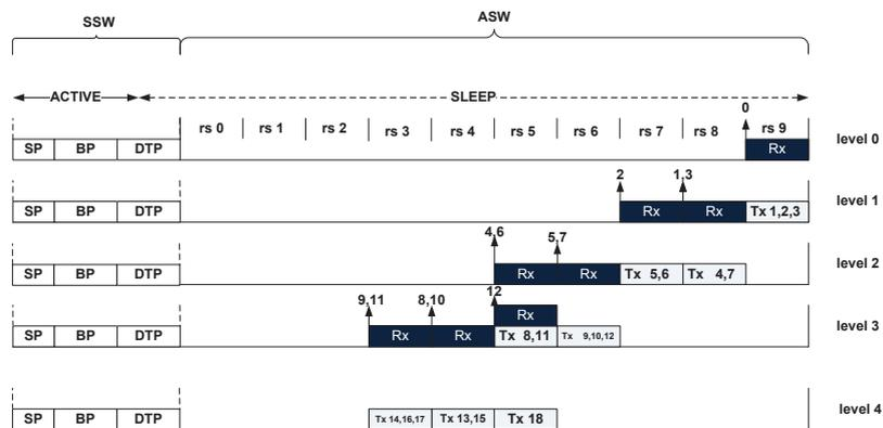
The first constraint ensures that, the slot assignment procedure will never select the same slot for two interfering receiver at the same level and hence, the simultaneous reception of two nodes at the same level must be interference free, assuming the interference might occur only for the transmission by the next lower level nodes. (refer to the definition of interfering-receiver).
