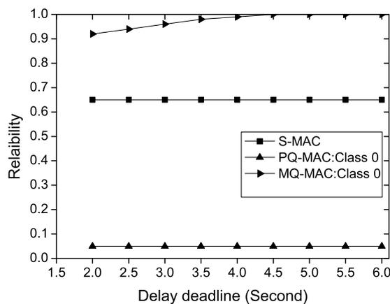
of delay deadline since, the operational cycle length of those protocols are always fixed. However, increase in the delay deadline also increases the reliability for the Class 0 traffic in MQ-MAC, due
