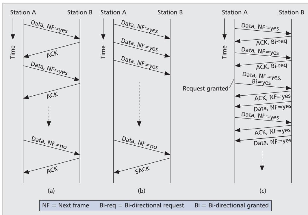
**Figure 5.** Typical Burst Mode scenarios for IEEE 1901 devices: a) uni-directional bursting with an immediate ACK policy; b) uni-directional bursting with a selective ACK policy; and c) bi-directional bursting.
