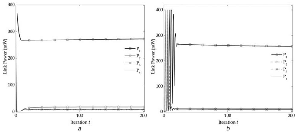
**Fig. 2** Convergence of link powers at the PU outage probability 10%
