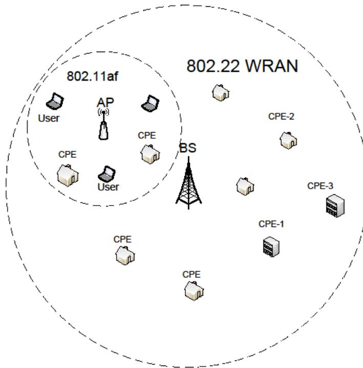
Figure 6: Heterogeneous coexistence scenario of different secondary networks
