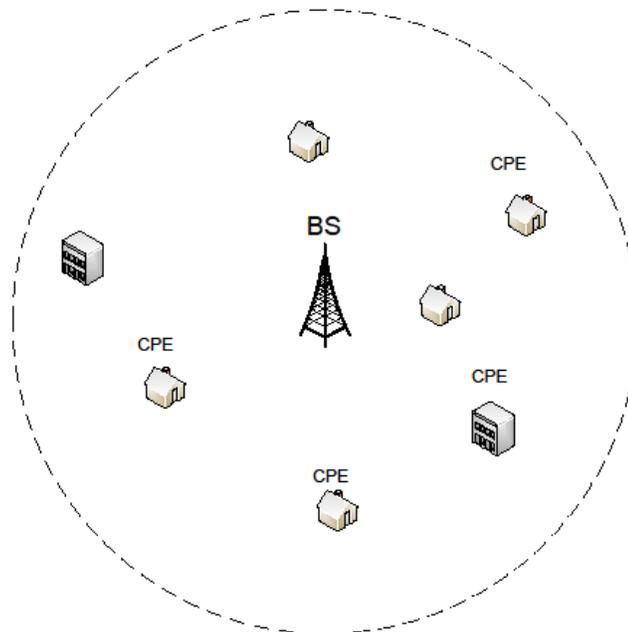
Figure 1: An IEEE 802.22 WRAN cell with a base station and CPEs
