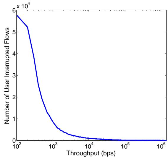
Fig. 2. Client interrupted connections with respect to throughput
