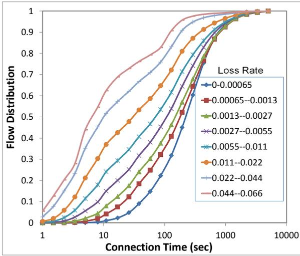
Fig. 3. Effect of Different Loss Rates on Connection Duration with Loss Rates between  $10^{-4}$  and  $10^{-2}$
