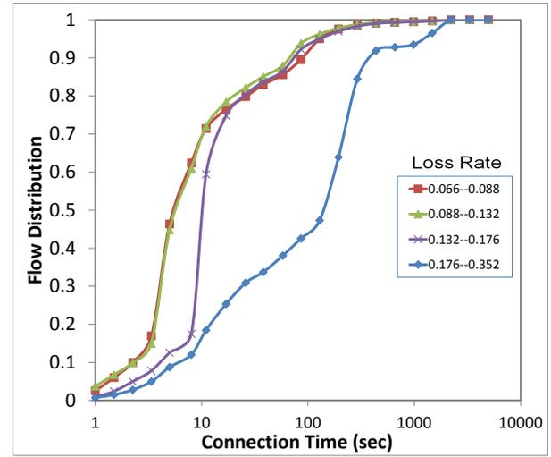
Fig. 4. Effect of Different Loss Rates on Connection Duration with Loss Rates between  $10^{-2}$  and  $10^{-1}$
