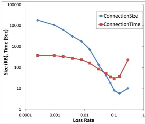
Fig. 5. Effect of loss rate on connection size and duration
