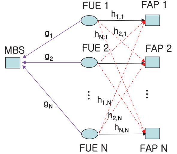
Fig. 2. Uplink transmission model.
