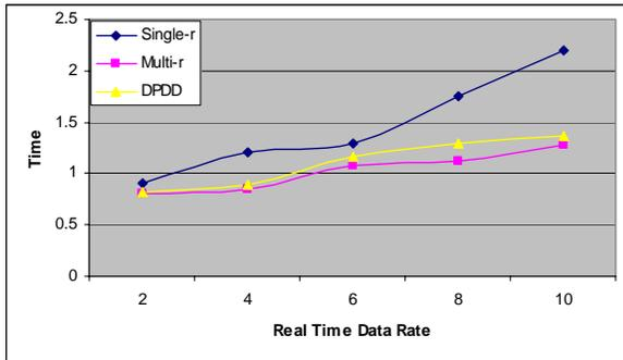
Fig. 6: Average delay per packet with different real-time data rates.
