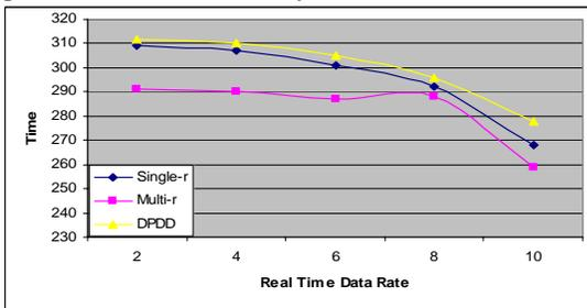
Fig. 7: Average lifetime of a node with different real-time data rates.
