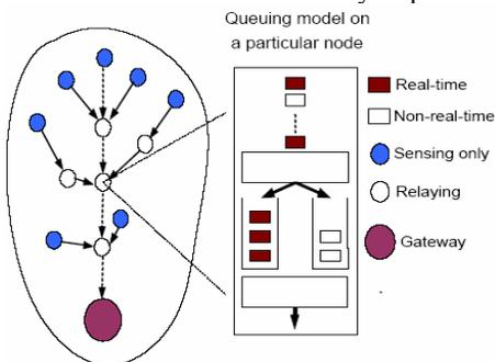
**Fig. 1:** Queuing model in a particular sensor node
