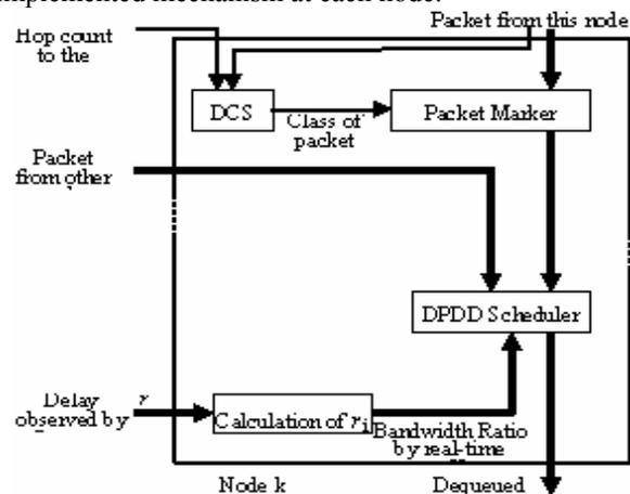
Fig. 5: End-to-end QoS assurance mechanisms based on DPDD and DCS
