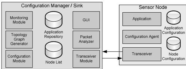
Figure 7. Information Flow and Architecture of the system
