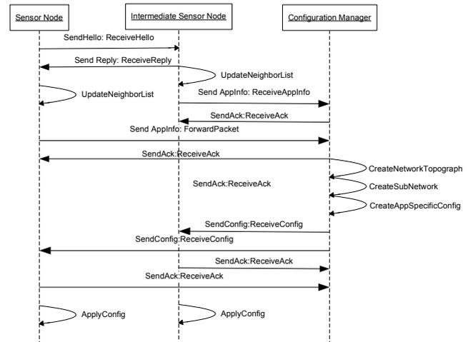
Figure 8. Sequence of message passing between the sensor nodes and the configuration manager.
