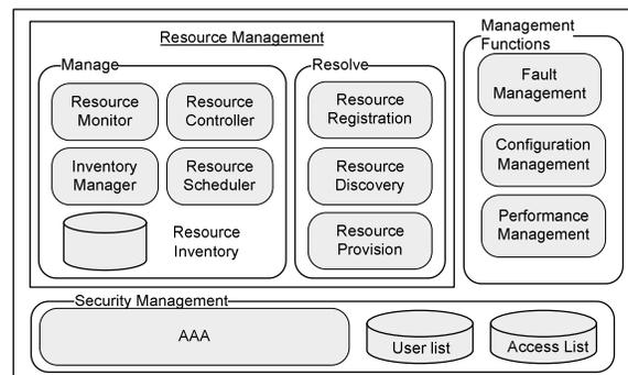
Figure 4: Modular diagram of a Resource Manager
