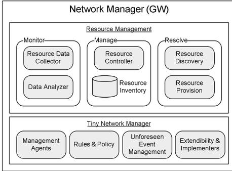
Figure 2: Network Manager at the WSN Gateway composing of TNM and Resource Management Module
