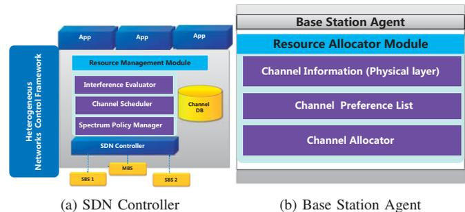
Fig. 1: SDN Controller and Base station agent
