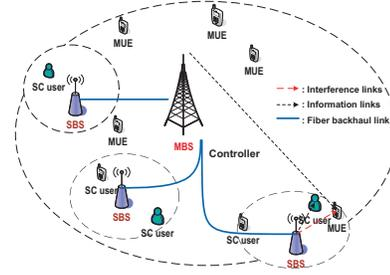
Fig. 2: Network Model. Solid line showing the downlink information links while dotted line showing the cross tier interference caused both by the MBS and SBS transmission.
