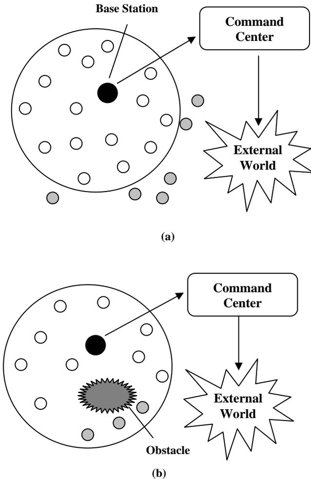
**Figure 1:** Sensor Deployment Scenario. a) Sensors out of transmission range of base station b) Sensors lose direct communication from base station due to obstacle
