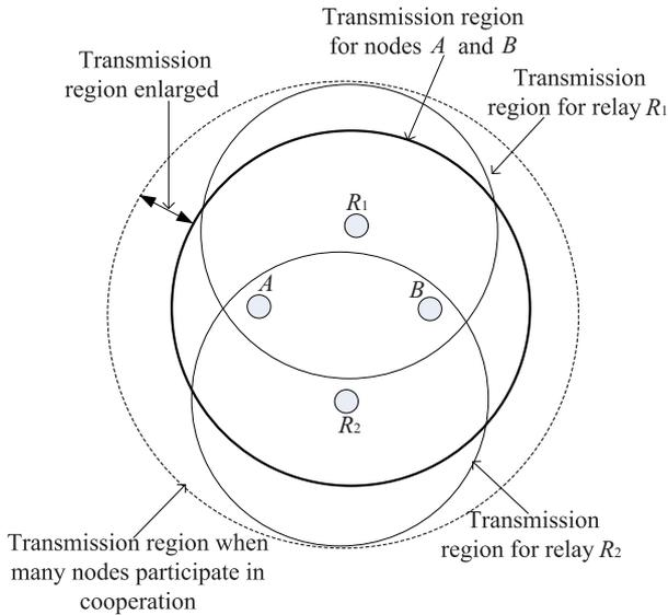
Fig. 3. Relay selection enlarges the transmission region.
