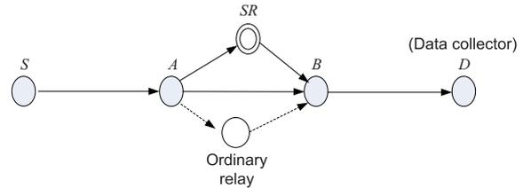
Fig. 4. Smart grid communication model.
