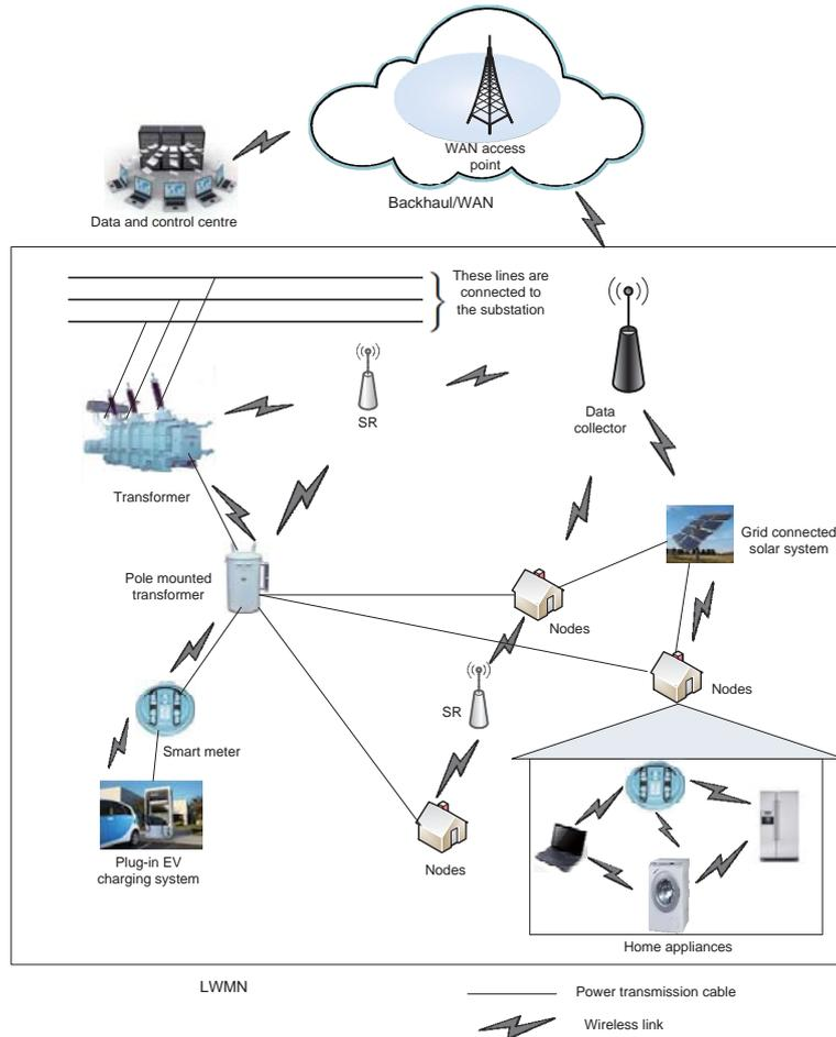
Fig. 1. Smart grid communication architecture based on an LWMN.
