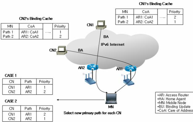
**Fig. 9.** Primary path selection for each correspondent node
