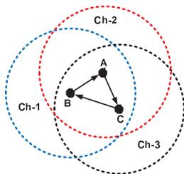
Fig. 2. Nodes are deployed on different channels and token is delivered to one node after another
