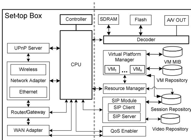
Figure 1. Modular design of the proposed Set-top box.
