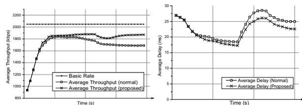
Figure 4. (a) Simulation results for average throughput and (b) simulation results for delay in milli-seconds, calculated at the STB for the data traffic between the service provider and the STB.
