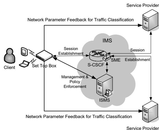
Figure 3. Feedback and signaling between the STB & ISMS (SME).
