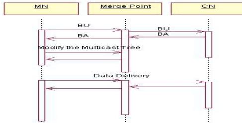
Fig. 6. Sequence Diagram of the Multicast Tree Scheme (MN as Sender)
