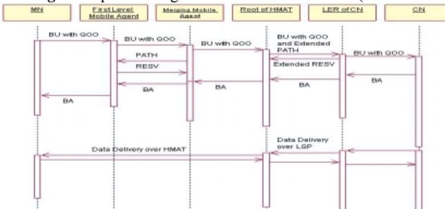
Fig. 8. Sequence Diagram of the HMAT Scheme (MN as Receiver)
