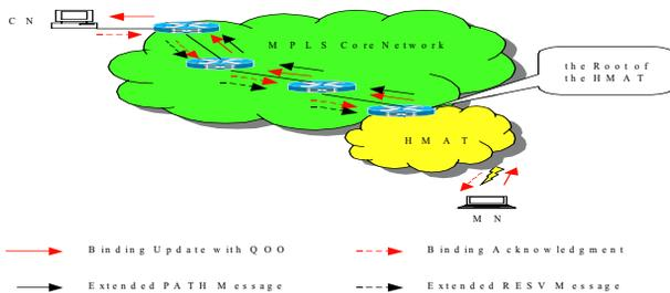
Fig. 3. Smooth Handoff Support in MPLS Core Network
