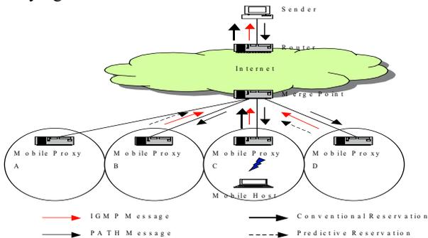
**Fig. 1.** RSVP Mobility Based on Multicast Tree
