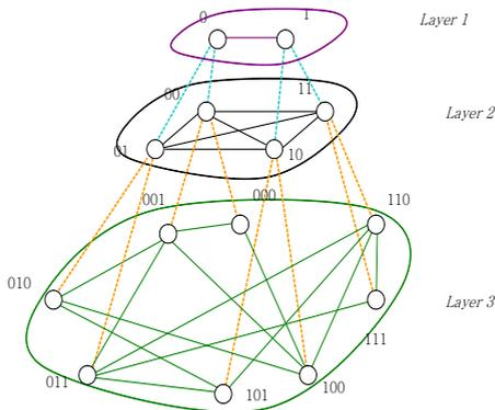
**Fig. 1.** A 3-layer hierarchical architecture. Node 01 (layer 2) is parent of two nodes 010 and 011 (layer 3) but is one of two children of node 0 (layer 1)
