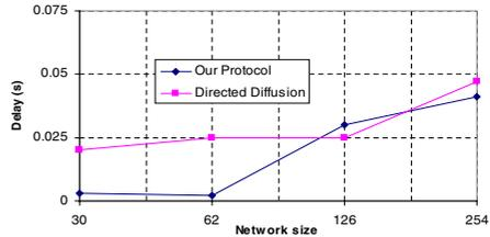
**Fig. 7 b.** Average end-to-end delay as a function of network size
