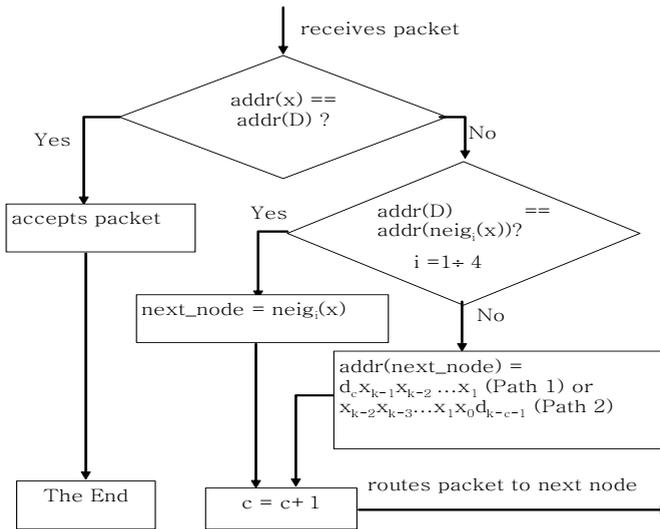
**Fig. 3.** Operations of node x.  $addr(x)$ ,  $neig_i(x)$ , and D present address,  $i^{th}$  neighbor of node x, and destination respectively
