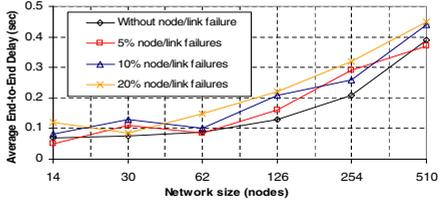
**Fig. 5 b.** Average end-to-end delay as a function of node/link failure as network size changes
