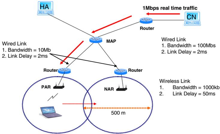
Fig. 7. Simulation network architecture
