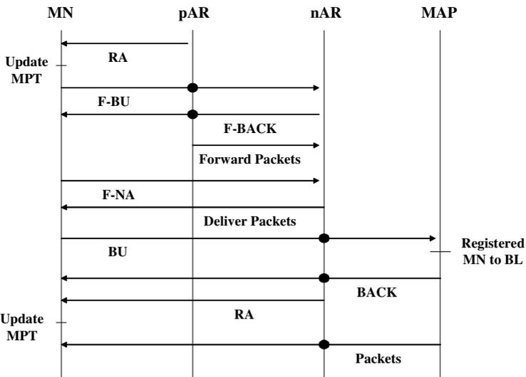
Fig. 6. The message sequence diagram of FH-Zone handover mechanism
