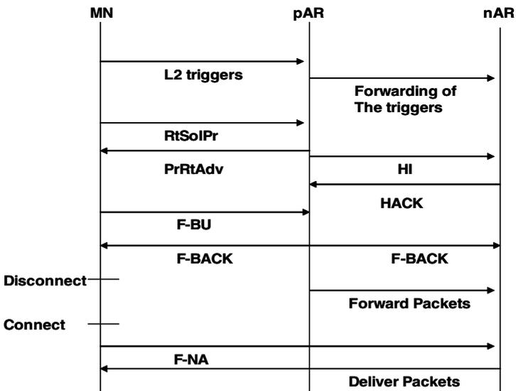
Fig. 2. The message sequence diagram of anticipated handover mechanism
