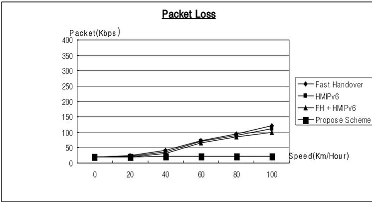
Fig. 10. Packet loss (overlap region: 20m, single user)
