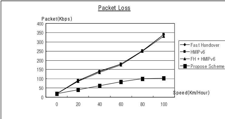
Fig. 9. Packet loss (overlap region: 50m, multiple users(5) )
