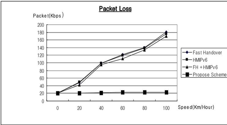
Fig. 8. Packet loss (overlap region: 50m, single user )
