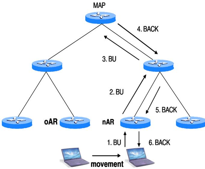
Fig. 1. Hierarchical Mobile IPv6 Operation
