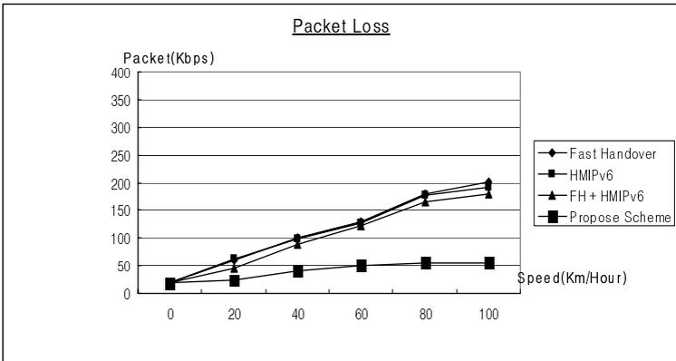
Fig. 11. Packet loss (overlap region: 20m, multiple users(5) )
