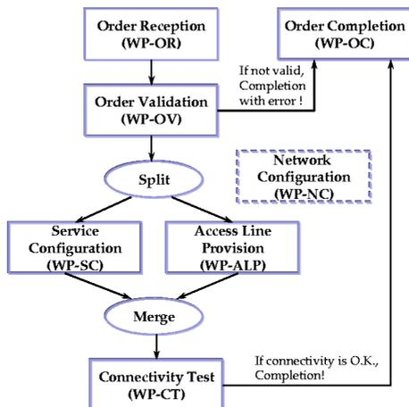
**Fig. 5.** A workflow for providing BGP/MPLS VPN service
